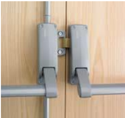
F412 09 001 Double Door set comprising a Panic Bar with Vertical Rods for the fixed leaf, and a Panic Latch Bar on the moving leaf
