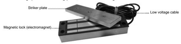
The electromagnet is usually attached rigidly to the door frame, and the striking plate is attached flexibly to the door. When the door is closed, the striking plate is close enough to be attracted, and held in position, by the electromagnet.
