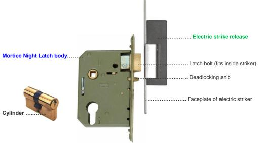
The cylinder operated latching mortice lock shown above has a deadlocking feature, which is activated whenever the deadlocking snib is depressed by contact with the faceplate of the electric striker. (The deadlocking **snib must NOT enter the striker**; it must ride **ON** the faceplate). This action deadlocks the latch, and enables the latch to resist being forced back.
