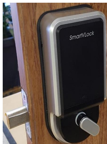
Inside view showing thumbturn for exit
